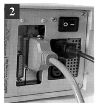
Plug a good quality, screened Centronics Interface cable into this socket and secure the wire latches. Plug the other end into the Printer connector of your PC (LPT1 or LPT2)
